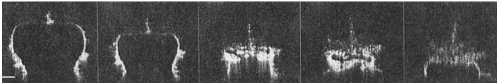
FIGURE 17. Second bubble collapse at \gamma = 1.66 and R_{\max} = 3.3\text{ mm} . Series taken with spatial filtering at 20\,000\text{ frames/s} . The location of the solid boundary is indicated by the white horizontal bar in the left frame. Frame size 4.5\text{ mm} \times 5\text{ mm} .
